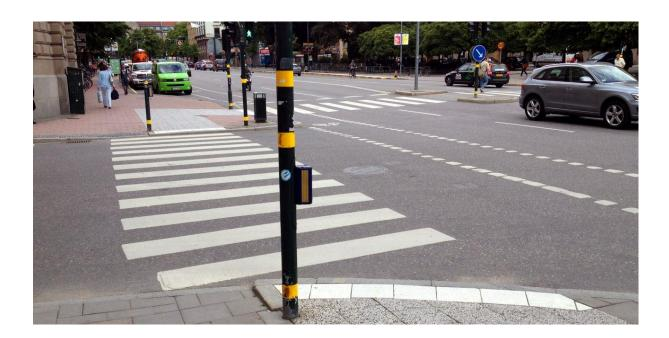
A ramp between street level and walkway on one side of the post and retained edge for orientation on the other side of the post is an elegant solution.
